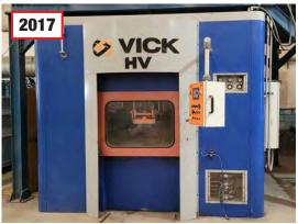
2017 VICK MODEL HV-3 3 STATION ROTARY COLD BOX CORE MACHINE, 15 TO 25 LITER CAPACITY WITH SAND MIXER, RESIN HEATER, SCRUBBER
