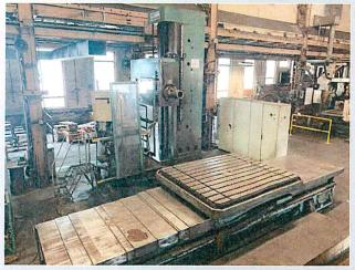
TOS VARNSDORF WHN13 CNC HORIZONTAL BORING MILL
